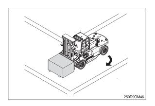
▲ Turn too sharp with a raised load and your truck can tip even at slow speeds. Travel with a load raised only when removing or depositing a load.
